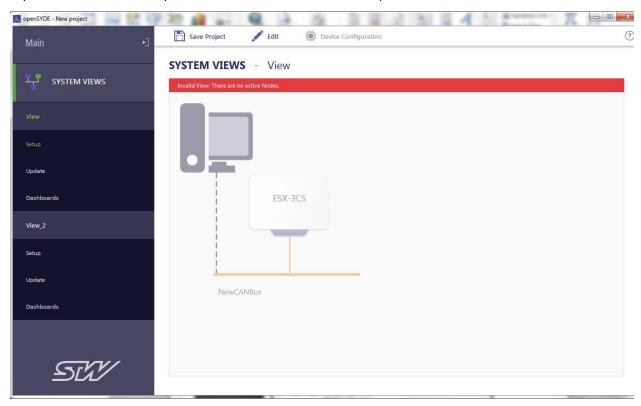
You will need to enable the controller by selecting Edit and then clicking the check box on the controller.
