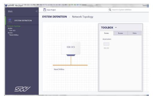
Double-click the controller to access its configuration parameters. You must enter the hex file to use for your controller in the Data Blocks section.
