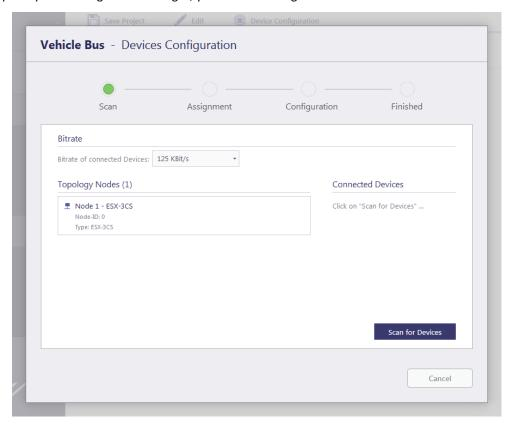
Scan for Devices, then turn on the controller. Drag the found devices into the appropriate system node, then select Configure devices
