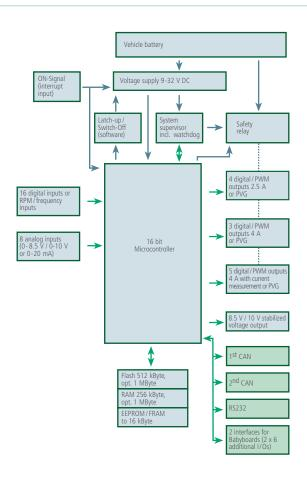
The freely programmable controller ESX® works independently as a measuring, driving or controlling device for sensor-actuator management and is capable of executing a number of separate or related tasks in real time.
